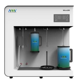
The AMI Micro 100 Series can accurately produce surface area and pore size results of powder materials. These instruments are divided into three types: A, B, and C, and the C type is configured with 1 torr or 0.1 torr high-sensitive pressure sensors and a turbo molecular pump with ultimate pressure of 10<sup>-8</sup> Pa. The C series can effectively perform an analysis of microporous materials such as: molecular sieve, catalyst, activated carbon, and other microporous materials.
